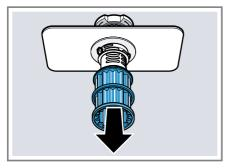
Press the locking catches 1 together and lift the coarse filter out 2.
