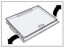
4. Lift the cover at the front ① and pull it out at the rear ②.
