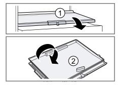
Press the fastenings for the lower cover outwards.
