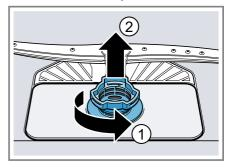
Pull down the micro filter to remove.
