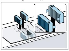
6. Insert the grease filter.
