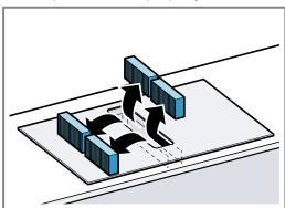
4. Insert two odour filters or acoustics filters into the left and right of the appliance and slide them forwards.
