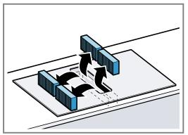
**4.** Insert two odour filters or acoustics filters into the left and right of the appliance and slide them forwards.
