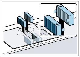
6. Insert the grease filter.
