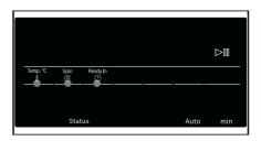
**Note:** The buttons are sensitive, they only need to be touched gently. If the button **Temp.** °C **(**,**Spin (**), **Ready In (**) is held down, the setting options are automatically scrolled through.
