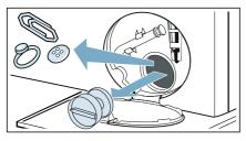
5. Refit and screw on the pump cover. The handle must be in a vertical position.
