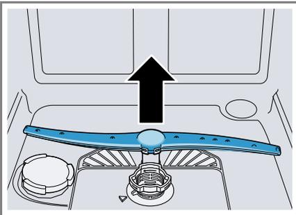
3. Check the outlet nozzles on the spray arms for blockages under running water and remove any foreign bodies.
