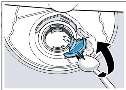
6. Lift the pump cover inwards at an angle and remove.
