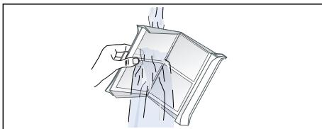
7. Dry the fluff filter, close it and reinser the two-part fluff filter.
