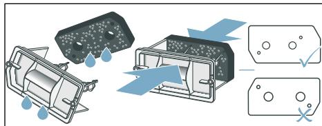
**Note:** Ensure that the filter mat is not misshapen, torn or clogged. Position the filter mat as shown above.
