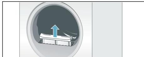
3. Remove the fluff from the recess in the fluff filter.
