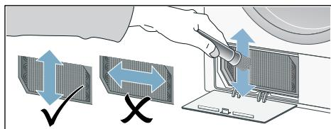
**Note:** Take care not to bend or damage the fins on the heat exchanger when cleaning it.
