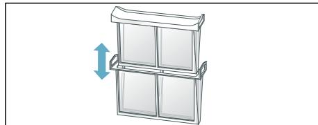
5. Open both filters and remove all the fluff.
