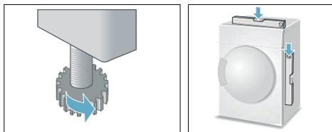
Incorrect alignment may cause high noise levels, vibrations and improper movement of the drum.
