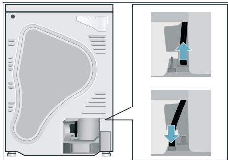
4. Take the drain hose from the accessories and secure it to the free connecting piece. Push the drain hose into the hose guide.
