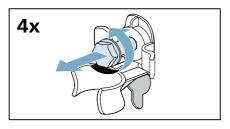
a) Remove the mains cable from the holders.
