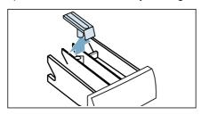
Clean the detergent dispenser tray and insert with water and a brush, and dry it. Clean the inside of the housing as well.
