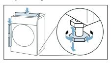
Tighten the lock nut against the housing. In doing so, hold the foot tight and do not adjust its height.
