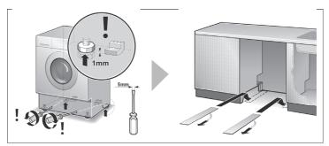
Slide sheets make it easier to slide the washing machine into the installation recess.
