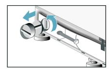
Replace the pump cover and screw firmly in place. Place the kick panel in the 4 clip-in slots and secure to the housing using the lock pins.
