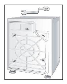
1. Unscrew all screws using the spanner supplied.
