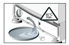
4. Carefully unscrew the pump cover; residual water may leak out. Clean the pump housing and remove any foreign objects. The impeller in the drain pump must be able to rotate.
