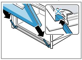
5. Close the locking levers on the left- and right-hand hinges.
