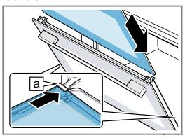
**6.** Push the inner pane upwards until it is in the left-and right-hand retainers a.
