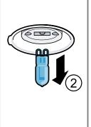
Insert the new halogen lamp and press it firmly into the socket.
