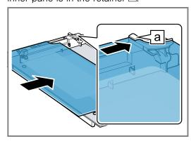
2. Push the inner pane upwards until it is in the leftand right-hand retainers a.
