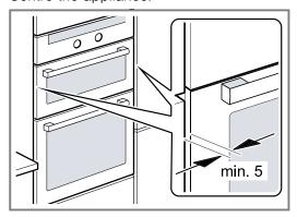
There must be an air gap of at least 5 mm between the appliance and adjacent unit fronts.
