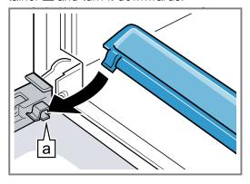
Slide the intermediate pane into the left- and righthand retainers a.
