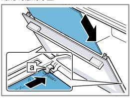
**4.** Push the intermediate pane upwards until it is in the left- and right-hand retainers a.
