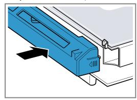
4. Slide the appliance door straight onto the two hinges. Slide the appliance door on as far as it will go. When doing so, ensure that the hinges are inserted into the correct opening.
