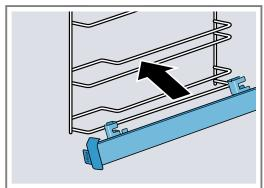
2. Push the retainer a in between the lower and the upper bar.
