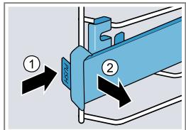
**3.** Pull the rail out towards the front until the retainer at the back unhooks.
