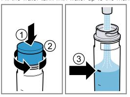
4. Press on the water tank lid ① and screw it on ②.
