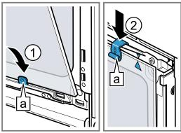
**4.** Attach the front pane downwards into the left- and right-hand retainers **a** ①.
