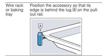
**Note:** The pull-out rails lock in place when they are fully pulled out. Gently push the pull-out rails back into the cooking compartment.
