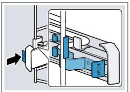
2. Keep the **PUSH** tab pushed back ① and swing the rail outwards ②.
