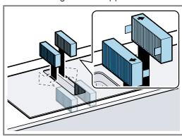
6. Insert the grease filter.
