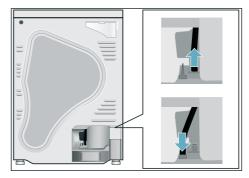
Take the drain hose from the accessories and secure it to the free connecting piece. Push the drain hose into the hose guide.
