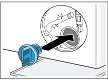
5. Screw on the pump cap.
