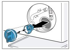
2 Clean the interior, the thread on the pump cap and the pump housing.
