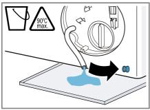
9. Firmly press on the sealing cap.
