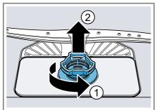
Pull down the micro filter to remove.
