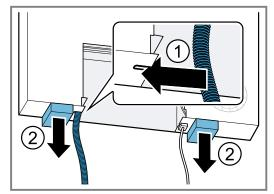
3. Note: To ensure that the appliance is not yet fully inserted into the cut-out, place a slat below the short side of the appliance in each case.
