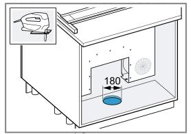
**7.** Slide the fan box into the guide, connect the pipework and screw the fan box tightly back in place.
