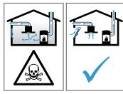
Always ensure adequate fresh air in the room if the appliance is being operated in exhaust air mode at the same time as a room-air-dependent heat-producing appliance is being operated.
