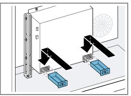
16.Plug the cables into the fan box.
