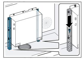
**12.Note:** If an appliance measuring 90 cm is installed in a unit with a width of 90 cm, skip the next two installation steps and follow the instructions in the additional accessory pack.
