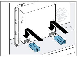
14. Plug the cables into the fan box.
