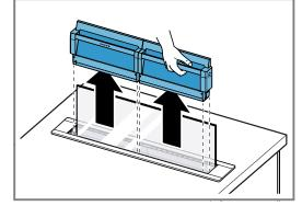
Insert the grease filter into the grease filter cartridges.
