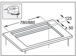
The angle between the cut surface and the worktop must be 90°.
