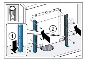
10. Screw the rails onto the bottom of the unit.
