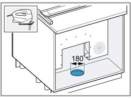
6. Slide the fan box into the guide, connect the pipework and screw the fan box tightly back in place.
