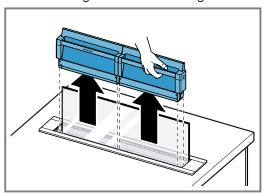
**3.** Insert the grease filter into the grease filter cartridges.
