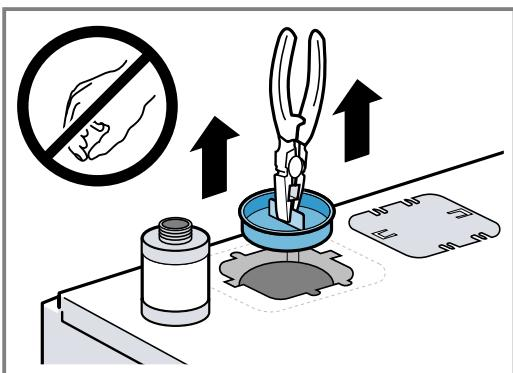
3. Secure the transport lock to the rear of the appliance for further use.
