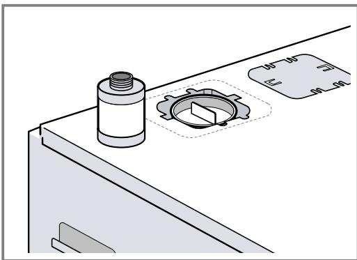
2. Remove the transport lock for the pump from the top of the appliance.
