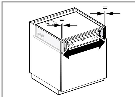
5. To check the tilt protection, open the drawer carefully.
