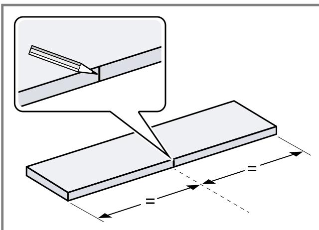
1. Measure the width of the fitted unit and mark the centre of the intermediate floor.
