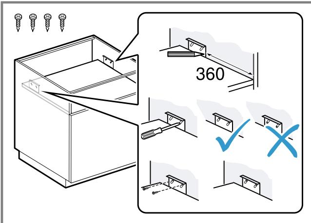
2. Use the installation aid to secure the mounting bracket to the unit.
