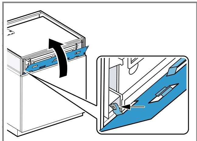
4. Check whether the front panel is mounted straight.
