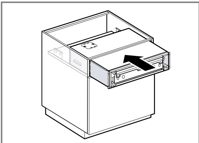
3. If the appliance cannot slide in, adjust the height of the tilt protection brackets. To do this, undo the screws and push the tilt protection brackets upwards.
