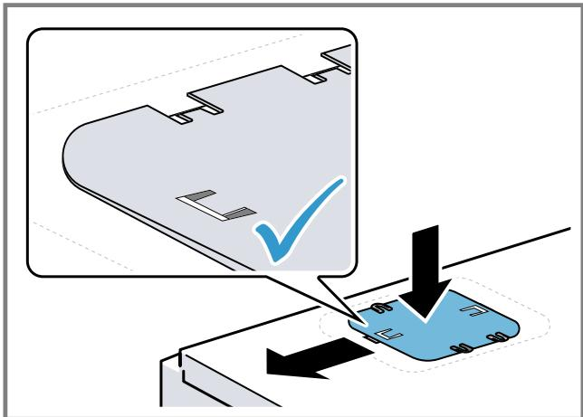
6. **⚠️ WARNING – Risk of tipping!** After removing the transportation lock, the drawer may open and the appliance may tip over.
