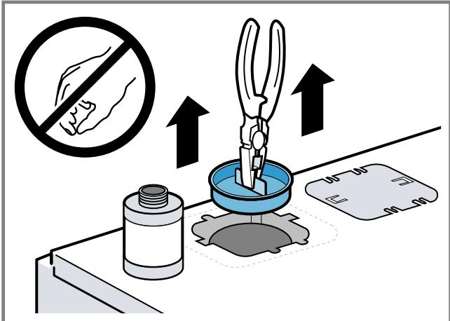
3. Secure the transport lock to the rear of the appliance for further use.
