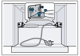
2. Appliance width 90 cm: Pull the filter pull-out out completely towards the front. Also use two screws each on the left and right to screw the appliance to the side upper cabinets from below.
