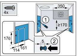
**8.** Screw in the four enclosed screws for the angle bracket up to 5 mm.
