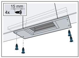
**3.** Adjust the wall closing strip to the clearance between the appliance and the wall.
