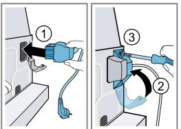
Screw the two angle brackets to the appliance. Note the position of the screws. Screw in the screws until 8 mm of the threaded section is still protruding.
