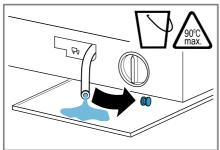
8. Firmly press on the sealing cap.
