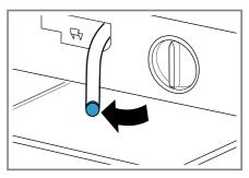
Insert the drain hose into the holder.
