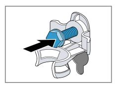
4. Insert the power cord into the holder 1 and tighten all four screws for the transit bolts with a WAF 13 wrench 2.
