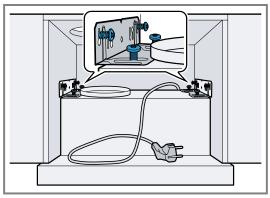
2. Appliance width 90 cm: Pull the filter pull-out out completely towards the front. Also use two screws each on the left and right to screw the appliance to the side upper cabinets from below.
