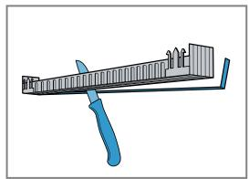
4. Snap the wall closing strip into the holders.
