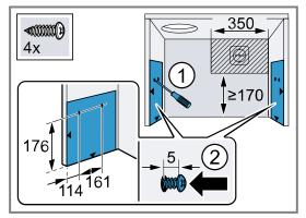
8. Screw in the four enclosed screws for the angle bracket up to 5 mm.
