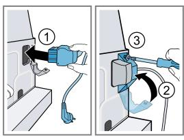
4. Screw the two angle brackets to the appliance. Note the position of the screws. Screw in the screws until 8 mm of the threaded section is still protruding.
