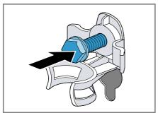
4. Insert the power cord into the holder ① and tighten all four screws for the transit bolts with a WAF 13 wrench ②.
