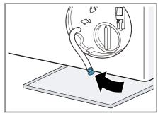
10.Insert the drain hose into the holder.
