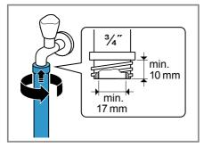
**3.** When connecting to a 21 mm = 1/2" tap, first fit the adapter with a sealing washer.
