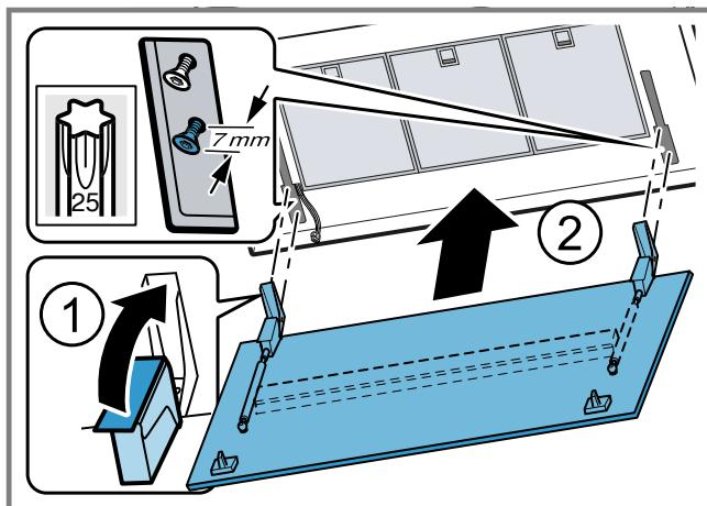
3. Tighten the fastening screws on the hinges.
