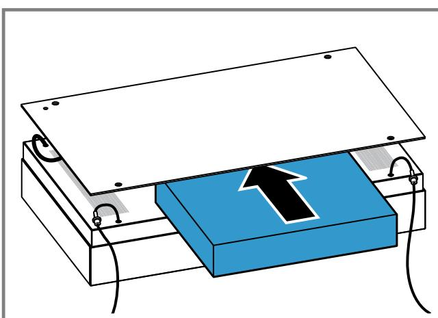
5. Thread the cables through the openings of the frame cover.
