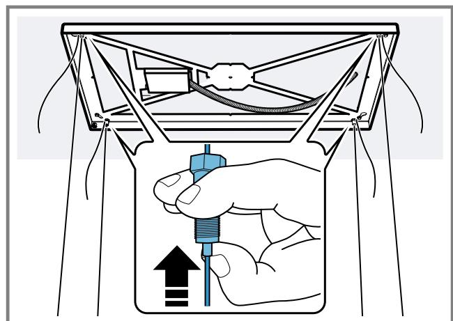
15. Thread the cables out of the frame cover.
