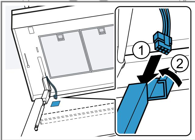
5. Close the cover on the cable duct.
