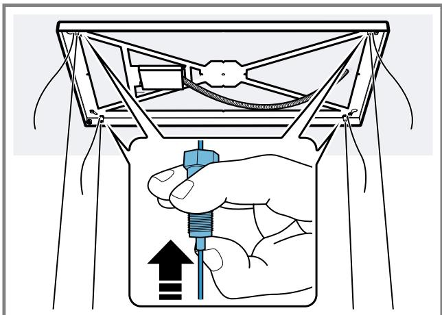
11. Thread the four enclosed cable clamps and secure in place approx. 20 mm in front of the cable tensioner.
