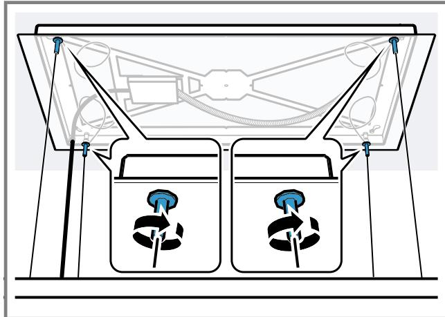
Do not use a tool to avoid damaging the frame cover.
