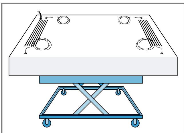
Do not place the appliance on the grease filters as these could be damaged.
