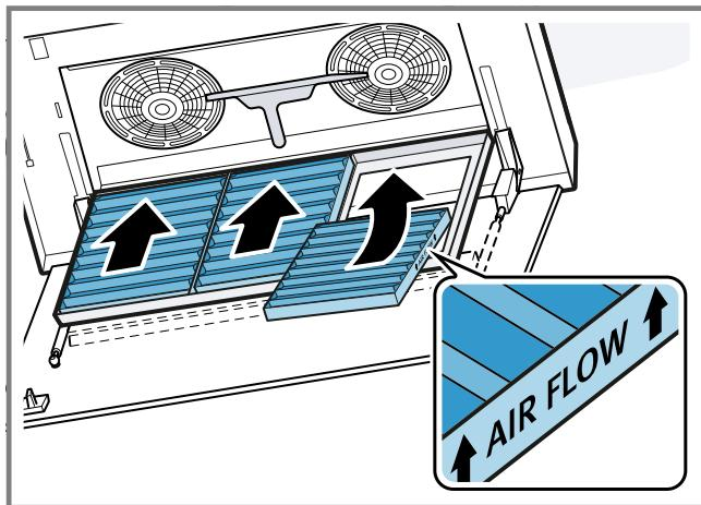
Insert the odour filter in the correct direction.
