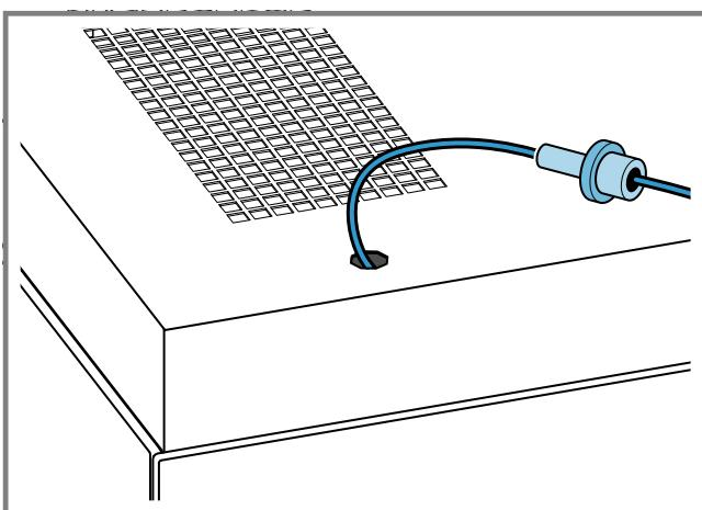
Do not insert the lock nuts into the openings to avoid damaging the appliance's limit switch.
