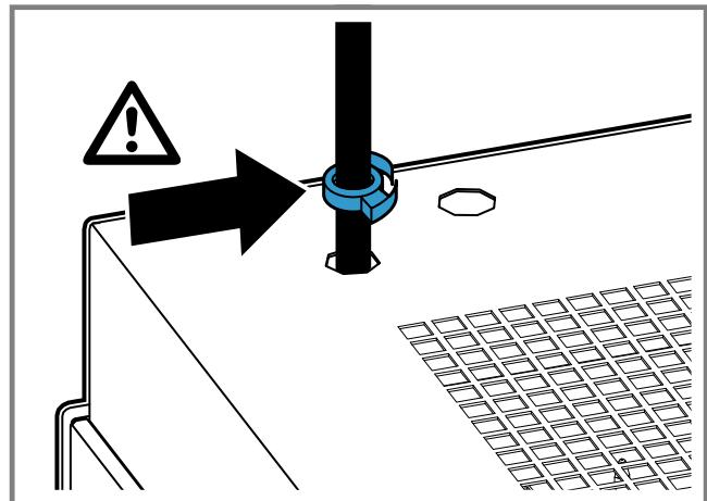
12. Remove the on-site cable from the terminal plug and remove the protective tube.
