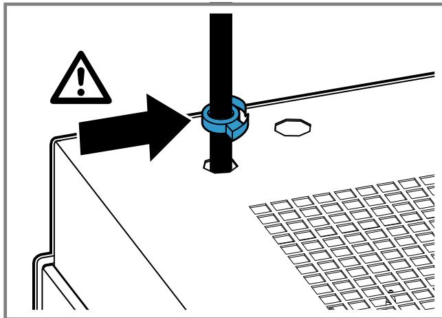
**17.** Remove the diagonally opposite screws on the frame.
