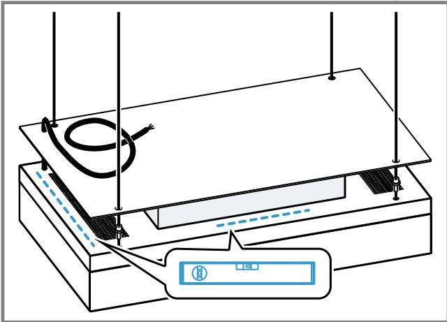
**13.** Remove the protective film from the appliance. Carefully remove the protective film around the cables so that the appliance's limit switch is not damaged.
