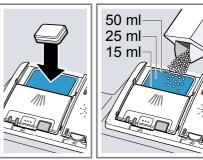
If you are using tablets, one is enough. Insert the tablets in a horizontal position.
