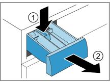
3. Pull out the insert upwards.
