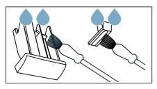
4. Fit the insert and lock it in place (push the cylinder onto the guide pin).
