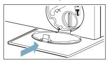
**Note:** To prevent unused detergent from flowing straight into the drain during the next wash: Pour 1 litre of water into dispenser II and start the **Drain** programme.
