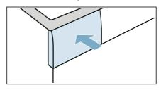
**Note:** Leave the detergent drawer open so that any residual water can evaporate.
