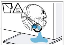
9. Firmly press on the sealing cap.
