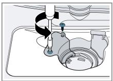
6. Pull up and remove the pump cover.
