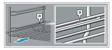
When inserting baking trays, make sure that the recess **a** is at the rear and is facing downwards. The sloping edge of the accessory **b** must be facing towards the appliance door.
