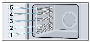
Always insert the accessory between the two guide bars for a shelf position.
