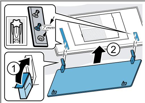
2. Mount the filter cover on the designated screws and push it backwards/forwards depending on the key hole opening into the narrow section.
