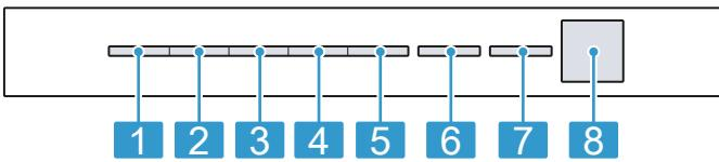
1 Fan setting 1/grease filter saturation display
