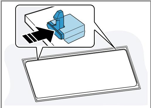
To prevent the filter cover from swinging down suddenly, hold onto the filter cover firmly with two hands.
