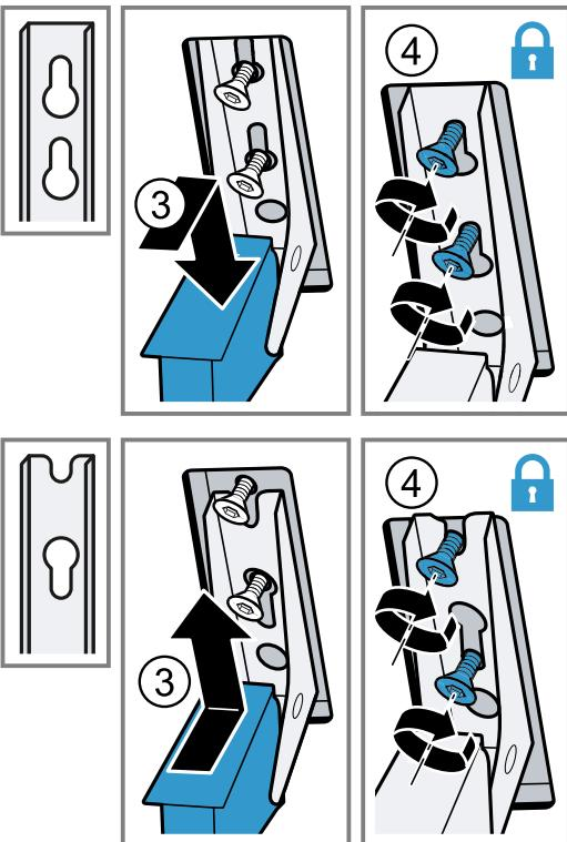
3. Tighten the fastening screws on the hinges.
