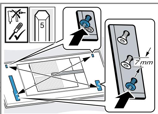
Retighten the screws if necessary.
