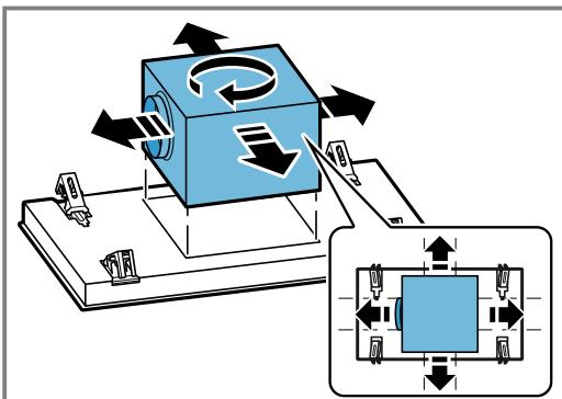
5. Push the fan box to the side and connect the appliance to the power supply.
