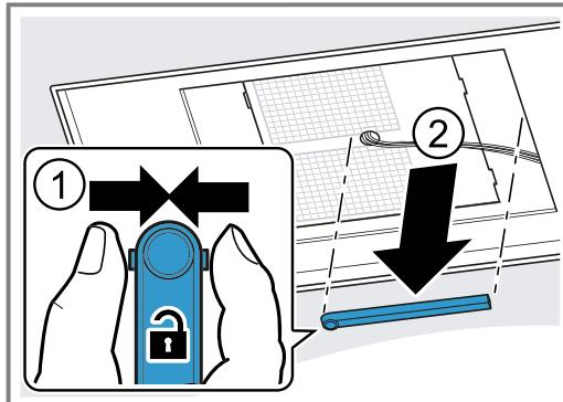
5. Disconnect the cable at the appropriate point.
