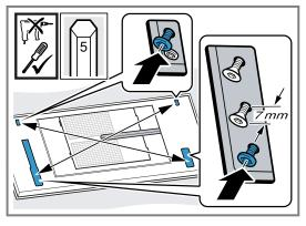
Retighten the screws if necessary.
