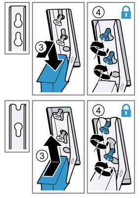
3. Tighten the fastening screws on the hinges.
