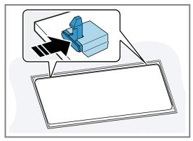
To prevent the filter cover from swinging down suddenly, hold onto the filter cover firmly with two hands.2. Open the filter cover by pulling it downwards.
