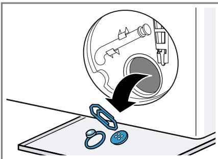
3. Make sure that the impeller in the drain pump can be turned.
