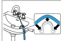
Drainage into a plastic pipe with rubber sleeve or into a gully.
