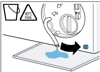
9. Firmly press on the sealing cap.
