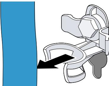
2. Unscrew ① and remove ② all four screws for the transit bolts with a WAF 13 wrench.
