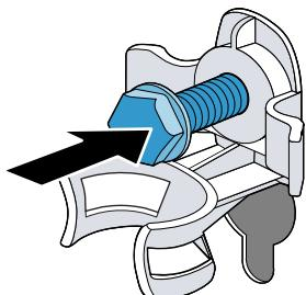
4. Insert the power cord into the holder ① and tighten all four screws for the transit bolts with a WAF 13 wrench ②.
