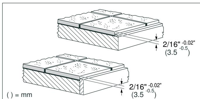
**Flush installation:** The appliance can be installed in the following temperature- and water-resistant countertops:
