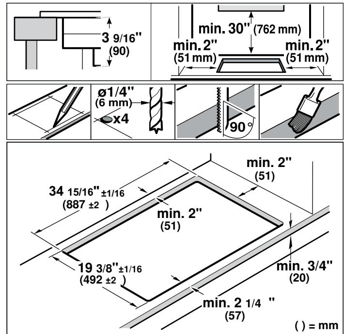
**Flush mounting:** Flush mounting into a countertop is possible.
