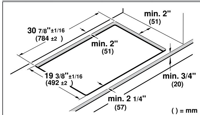
**Flush mounting:** Flush mounting into a countertop is possible.
