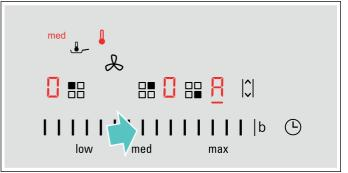
The function has now been activated. The I temperature symbol will remain lit until the frying temperature has been reached. An audible signal sounds and the temperature symbol goes out.
