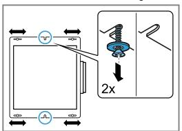
10. Align the motor block and tighten all of the screws.
