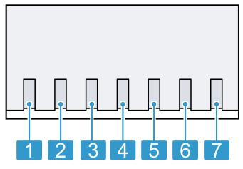
Fan setting 1 Fan setting 2 Fan setting 3 4 Intensive mode Fan run-on Intermittent mode Saturation indicator
