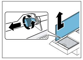
3. Remove the grease filters.
