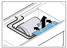
6. Loosen both plug connections and release the cables from the cable holders.
