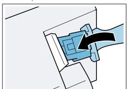
14. Insert the motor into the motor block 1 and screw it in tightly 2.
