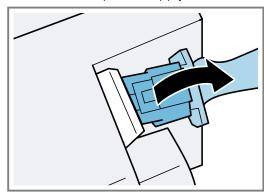
10. Remove the air pipe connector.
