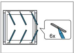
**4.** Screw in one of the two middle screws, but do not screw it in completely.
