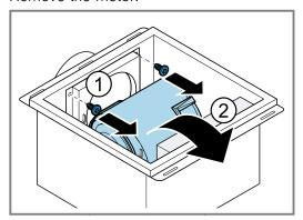
**9.** Disconnect the power supply from the motor.
