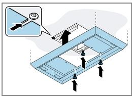
17. Insert both plug connections and hook on the cables.
