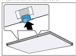
To prevent the filter cover from swinging down suddenly, hold onto the filter cover firmly with two
