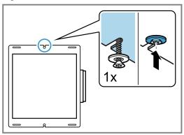
**8.** Screw in the remaining four screws loosely; do not tighten them fully.
