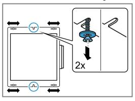
10. Align the motor block and tighten all of the screws.
