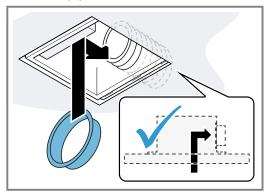
**13.** Insert the power cable into the motor.
