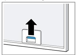
**4.** Remove the grease filters from the holders. To prevent grease from dripping, hold the grease filter horizontally.
