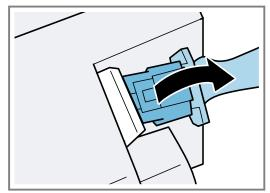
10. Remove the air pipe connector.
