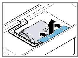
6. Loosen both plug connections and release the cables from the cable holders.
