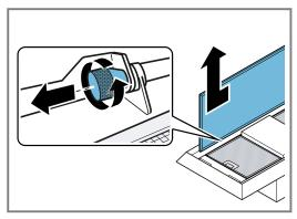
3. Remove the grease filters.
