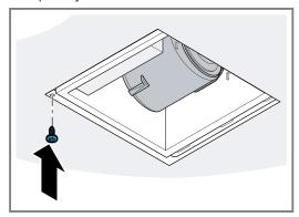
16. Hook the view frame onto the elongated hole and tighten all of the screws.
