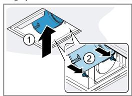
15. Secure the screw for the elongated hole in the view frame on the motor block, but do not screw it in completely.
