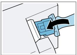
**14.** Insert the motor into the motor block ① and screw it in tightly ②.
