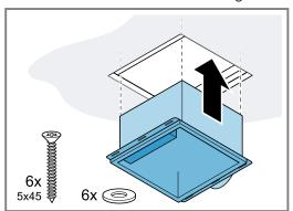
3. Align the motor block, mark the drill holes, and set the motor block down again.
