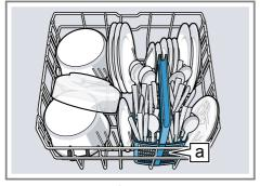
Cutlery basket a1 Large plates up to a diameter of 31/34 cm<sup>1</sup> can be arranged as shown.
