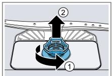
Pull down the micro filter to remove.
