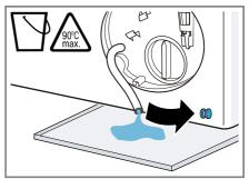
9. Firmly press on the sealing cap.
