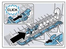
Check that the mounts are in the correct position.
