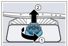
3. Pull down the micro filter to remove.
