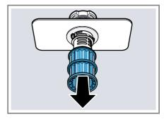
4. Press the locking catches 1 together and lift the coarse filter out 2).
