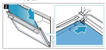
3. Press down on the top of the intermediate glass panel (fig. 3).
