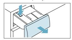
**4.** Press the pump unit insert and remove it.
