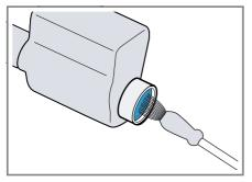
**3.** Connect the water inlet hose and check for leaks.
