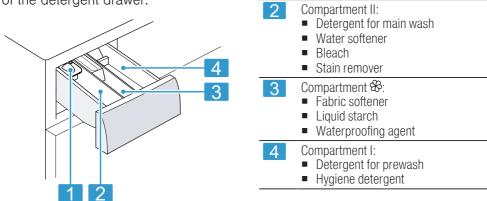
Measuring aid for liquid detergent → "Using a measuring aid for liquid
