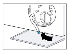
10.Insert the drain hose into the holder.
