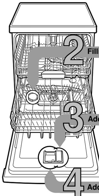
**2 Filling the salt dispenser** Dissolves limescale (not necessary when set to 0!) ...
